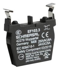
Schmersal contact block, plastic, (1) N.O./(1) N.C. contact(s), mounting position 3. For use with N series pushbuttons and switches. Not suitable for E-stop devices NDRZ50RT/ NDRZ50RT-2905-1.
