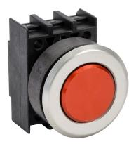
Schmersal pushbutton, IP65, 30mm, momentary, operator only, plastic base, metal bezel, Operator: red, flush, 29.5mm, round, metal. Requires contact blocks.
