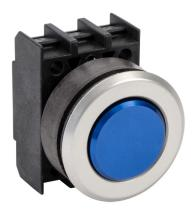
Schmersal pushbutton, IP65, 30mm, momentary, operator only, plastic base, metal bezel, Operator: blue, flush, 29.5mm, round, metal. Requires contact blocks.
