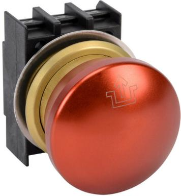
Schmersal emergency stop pushbutton, IP65, 30mm, push-lock pull-reset, operator only, plastic base, metal bezel, Operator: red, mushroom, 40mm, round, metal. Requires contact blocks.
