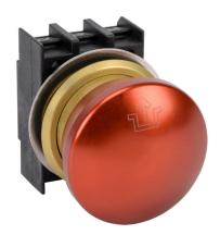
Schmersal emergency stop pushbutton, IP65, 30mm, push-lock pull-reset, operator only, plastic base, metal bezel, Operator: red, mushroom, 40mm, round, metal. Requires contact blocks.
