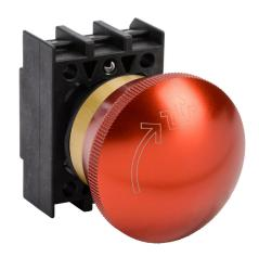
Schmersal pushbutton, IP65, 22mm, push to lock, twist and pull to reset, operator only, plastic base, plastic bezel, yellow, Operator: red, mushroom, 40mm, round, aluminum, operator text "push/pull/twist". Purchase contact blocks separately.
