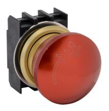
Schmersal emergency stop pushbutton, IP65, 30mm, twist-torelease, operator only, plastic base, metal bezel, Operator: red, mushroom, 40mm, round, metal. Requires contact blocks and EFR spring element.
