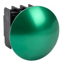
Schmersal pushbutton, IP65, 30mm, momentary, operator only, plastic base, metal bezel, Operator: green, mushroom, 55mm, round, metal. Requires contact blocks.
