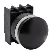
Schmersal pushbutton, IP65, 30mm, momentary, operator only, plastic base, metal bezel, Operator: black, mushroom, 40mm, round, metal. Requires contact blocks.
