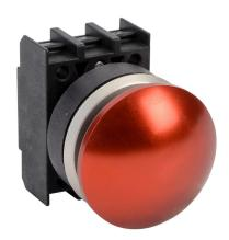
Schmersal pushbutton, IP65, 30mm, momentary, operator only, plastic base, metal bezel, Operator: red, mushroom, 40mm, round, metal. Requires contact blocks.
