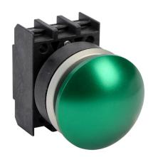
Schmersal pushbutton, IP65, 30mm, momentary, operator only, plastic base, metal bezel, Operator: green, mushroom, 40mm, round, metal. Requires contact blocks.
