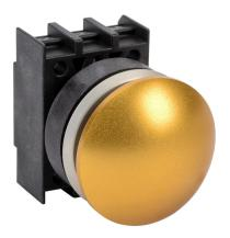
Schmersal pushbutton, IP65, 30mm, momentary, operator only, plastic base, metal bezel, Operator: yellow, mushroom, 40mm, round, metal. Requires contact blocks.
