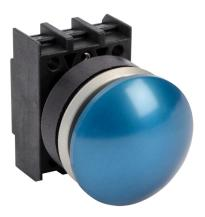
Schmersal pushbutton, IP65, 30mm, momentary, operator only, plastic base, metal bezel, Operator: blue, mushroom, 40mm, round, metal. Requires contact blocks.
