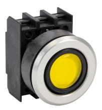
Schmersal pushbutton, IP65, 30mm, momentary, operator only, plastic base, metal bezel, Operator: yellow, flush, 29.5mm, round, glass. Requires contact and light blocks.
