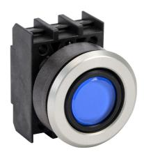
Schmersal pushbutton, IP65, 30mm, momentary, operator only, plastic base, metal bezel, Operator: blue, flush, 29.5mm, round, glass. Requires contact and light blocks.
