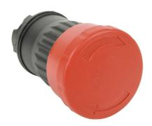
Comepi emergency stop pushbutton, IP65, 22mm, twist-to-release, operator only, thermoplastic base, thermoplastic bezel, Operator: red, mushroom, 40mm, mushroom, plastic, operator text "arrow". Requires ECX4029-2 mounting flange and ECX10x0N-2 contact block.
