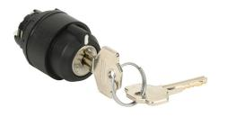
Comepi selector switch, IP65, 22mm, 2-position, maintained, key removable left position, operator only, thermoplastic base, thermoplastic bezel, Operator: black, key-operated, 30mm, round. Requires ECX4029-2 mounting flange and ECX10x0N-2 contact block.
