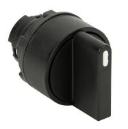
Comepi selector switch, IP65, 22mm, 3-position, maintained, operator only, thermoplastic base, thermoplastic bezel, Operator: black, knob, 30mm, round. Requires ECX4029-2 mounting flange and ECX10x0N-2 contact block.
