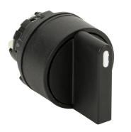
Comepi selector switch, IP65, 22mm, 2-position, maintained, operator only, thermoplastic base, thermoplastic bezel, Operator: black, knob, 30mm, round. Requires ECX4029-2 mounting flange and ECX10x0N-2 contact block.
