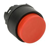
Comepi pushbutton, IP65, 22mm, momentary, operator only, thermoplastic base, thermoplastic bezel, Operator: red, extended, 30mm, round, plastic. Requires ECX4029-2 mounting flange and ECX10x0N-2 contact block.
