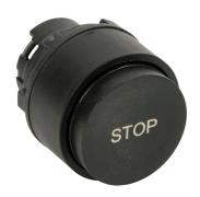
Comepi pushbutton, IP65, 22mm, momentary, operator only, thermoplastic base, thermoplastic bezel, Operator: black, extended, 30mm, round, plastic, operator text "STOP". Requires ECX4029-2 mounting flange and ECX10x0N-2 contact block.
