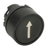
Comepi pushbutton, IP65, 22mm, momentary, operator only, thermoplastic base, thermoplastic bezel, Operator: black, flush, 30mm, round, plastic, operator text "down arrow". Requires ECX4029-2 mounting flange and ECX10x0N-2 contact block.
