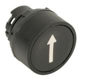
Comepi pushbutton, IP65, 22mm, momentary, operator only, thermoplastic base, thermoplastic bezel, Operator: black, flush, 30mm, round, plastic, operator text "up arrow". Requires ECX4029-2 mounting flange and ECX10x0N-2 contact block.
