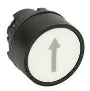
Comepi pushbutton, IP65, 22mm, momentary, operator only, thermoplastic base, thermoplastic bezel, Operator: white, flush, 30mm, round, plastic, operator text "up arrow". Requires ECX4029-2 mounting flange and ECX10x0N-2 contact block.
