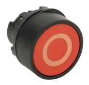
Comepi pushbutton, IP65, 22mm, momentary, operator only, thermoplastic base, thermoplastic bezel, Operator: red, flush, 30mm, round, plastic, operator text "(O)". Requires ECX4029-2 mounting flange and ECX10x0N-2 contact block.
