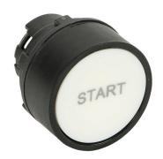
Comepi pushbutton, IP65, 22mm, momentary, operator only, thermoplastic base, thermoplastic bezel, Operator: white, flush, 30mm, round, plastic, operator text "START". Requires ECX4029-2 mounting flange and ECX10x0N-2 contact block.
