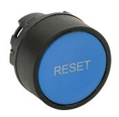
Comepi pushbutton, IP65, 22mm, momentary, operator only, thermoplastic base, thermoplastic bezel, Operator: blue, flush, 30mm, round, plastic, operator text "RESET". Requires ECX4029-2 mounting flange and ECX10x0N-2 contact block.
