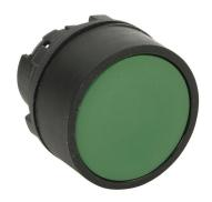
Comepi pushbutton, IP65, 22mm, momentary, operator only, thermoplastic base, thermoplastic bezel, Operator: green, flush, 30mm, round, plastic. Requires ECX4029-2 mounting flange and ECX10x0N-2 contact block.
