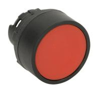
Comepi pushbutton, IP65, 22mm, momentary, operator only, thermoplastic base, thermoplastic bezel, Operator: red, flush, 30mm, round, plastic. Requires ECX4029-2 mounting flange and ECX10x0N-2 contact block.
