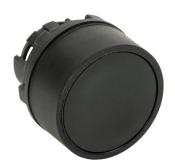
Comepi pushbutton, IP65, 22mm, momentary, operator only, thermoplastic base, thermoplastic bezel, Operator: black, flush, 30mm, round, plastic. Requires ECX4029-2 mounting flange and ECX10x0N-2 contact block.
