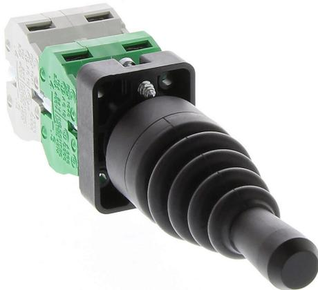
AutomationDirect selector switch, IP65, 22mm, 4-position, momentary, (4) N.O. contact(s), plastic base, plastic bezel, Operator: black, joystick, 30mm, round, plastic.
