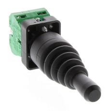
AutomationDirect selector switch, IP65, 22mm, 2-position, maintained, (2) N.O. contact(s), plastic base, plastic bezel, Operator: black, joystick, 30mm, round, plastic.
