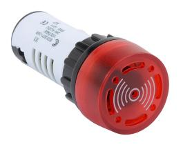
AutomationDirect audible alarm buzzer, 80 dB at 10cm, 2.8 kHz tone frequency, pulse tone(s), 24 VAC/VDC, permanent LED indicator(s), red, 22mm, panel mount, plastic housing, red, IP65.
