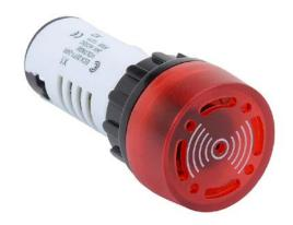
AutomationDirect audible alarm buzzer, 80 dB at 10cm, 2.8 kHz tone frequency, pulse tone(s), 24 VAC/VDC, permanent LED indicator(s), red, 22mm, panel mount, plastic housing, red, IP65.
