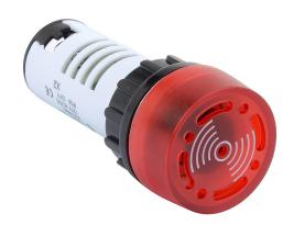
AutomationDirect audible alarm buzzer, 80 dB at 10cm, 2.8 kHz tone frequency, pulse tone(s), 120 VAC/VDC, permanent LED indicator(s), red, 22mm, panel mount, plastic housing, red, IP65.
