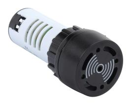
AutomationDirect audible alarm buzzer, 80 dB at 10cm, 2.4 kHz tone frequency, pulse tone(s), 24 VAC/VDC, 22mm, panel mount, plastic housing, black, IP65.
