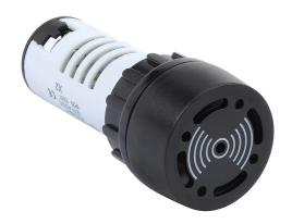
AutomationDirect audible alarm buzzer, 80 dB at 10cm, 2.4 kHz tone frequency, pulse tone(s), 120 VAC/VDC, 22mm, panel mount, plastic housing, black, IP65.
