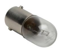
AutomationDirect bulb, incandescent, replacement, 24 VAC/VDC, T31/4 bayonet, 80 mA @ 24V. Package of 5. For use with GCX and ECX series pushbuttons, switches and indicators.
