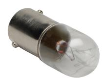
AutomationDirect bulb, incandescent, replacement, 6 VAC/VDC, T31/4 bayonet, 1.2W @ 6V. Package of 5. For use with GCX and ECX series pushbuttons, switches and indicators.
