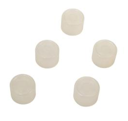
AutomationDirect protection cap, clear, 22mm, silicone. Package of 5. For use with GCX series extended or illuminated pushbuttons.
