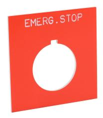
AutomationDirect jumbo legend plate, plastic, square, red field, red background, white engraved text, legend plate marking "EMERG. STOP". For use with 22mm pilot devices. O-ring included.
