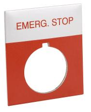
AutomationDirect jumbo legend plate, aluminum, rectangular, red field, silver background, red engraved text, legend plate marking "EMERG. STOP". For use with 22mm pilot devices. O-ring included.
