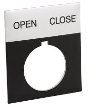
AutomationDirect jumbo legend plate, aluminum, rectangular, black field, silver background, black engraved text, legend plate marking "OPEN CLOSE". For use with 22mm pilot devices. O-ring included.
