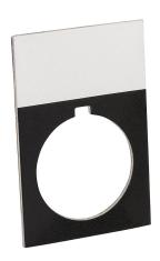
AutomationDirect legend plate, aluminum, rectangular, black field, silver background, legend plate marking "blank". For use with 22mm pilot devices. O-ring included.
