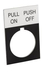
AutomationDirect legend plate, aluminum, rectangular, black field, silver background, black engraved text, legend plate marking "PULL ON PUSH OFF". For use with 22mm pilot devices. O-ring included.
