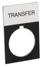
AutomationDirect legend plate, aluminum, rectangular, black field, silver background, black engraved text, legend plate marking "TRANSFER". For use with 22mm pilot devices. O-ring included.
