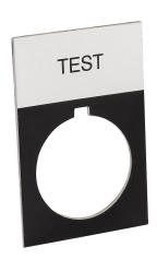
AutomationDirect legend plate, aluminum, rectangular, black field, silver background, black engraved text, legend plate marking "TEST". For use with 22mm pilot devices. O-ring included.
