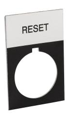
AutomationDirect legend plate, aluminum, rectangular, black field, silver background, black engraved text, legend plate marking "RESET". For use with 22mm pilot devices. O-ring included.
