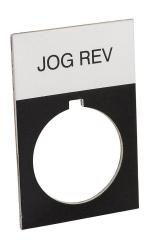
AutomationDirect legend plate, aluminum, rectangular, black field, silver background, black engraved text, legend plate marking "JOG REV". For use with 22mm pilot devices. O-ring included.
