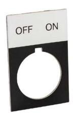
AutomationDirect legend plate, aluminum, rectangular, black field, silver background, black engraved text, legend plate marking "OFF ON". For use with 22mm pilot devices. O-ring included.
