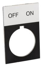
AutomationDirect legend plate, aluminum, rectangular, black field, silver background, black engraved text, legend plate marking "OFF ON". For use with 22mm pilot devices. O-ring included.
