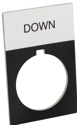
AutomationDirect legend plate, aluminum, rectangular, black field, silver background, black engraved text, legend plate marking "DOWN". For use with 22mm pilot devices. O-ring included.
