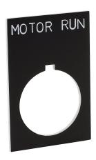
AutomationDirect legend plate, plastic, rectangular, black field, black background, white engraved text, legend plate marking "MOTOR RUN". For use with 22mm pilot devices. O-ring included.
